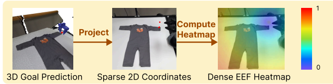
Fig. 7: End-effector heatmap generation for goal conditioning. Predicted 3D keypoints are projected to 2D coordinates, and then converted to dense distance heatmaps that encode spatial proximity to each keypoint.
